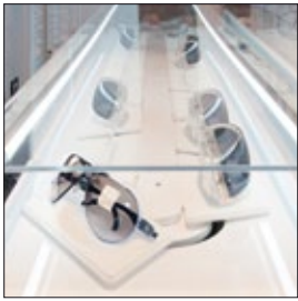
Plateaux se déplacent sans interruption sur un tapis roulant ovale. Shelves move continuously on an oval track.
